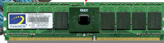
DRAM 晶片:Wire Bonding 模組:PCB
